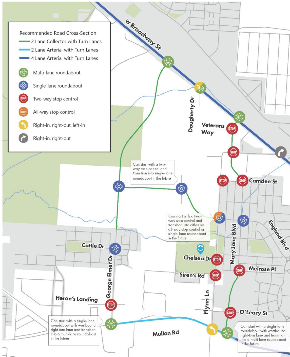
Figure 10 Intersection Control & Roadway Cross-Section Recommendations (2050)
