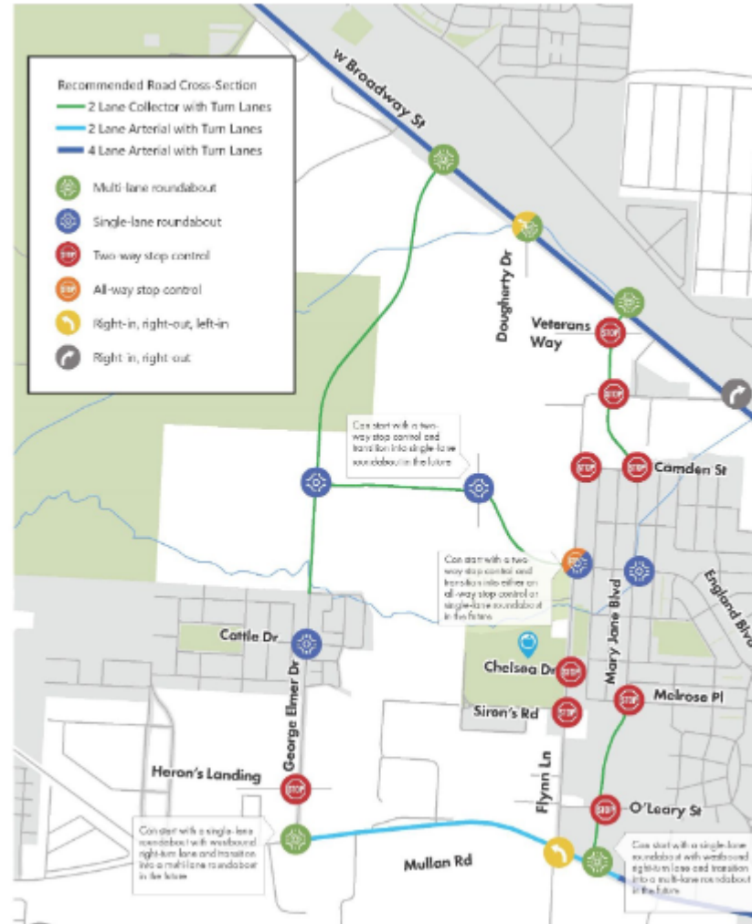
Figure 10 Intersection Control & Roadway Cross-Section Recommendations (2050)
